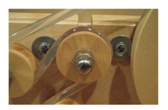
With the tool supplied remove the M6 machine screws and washers on both sides of the carder frame.
